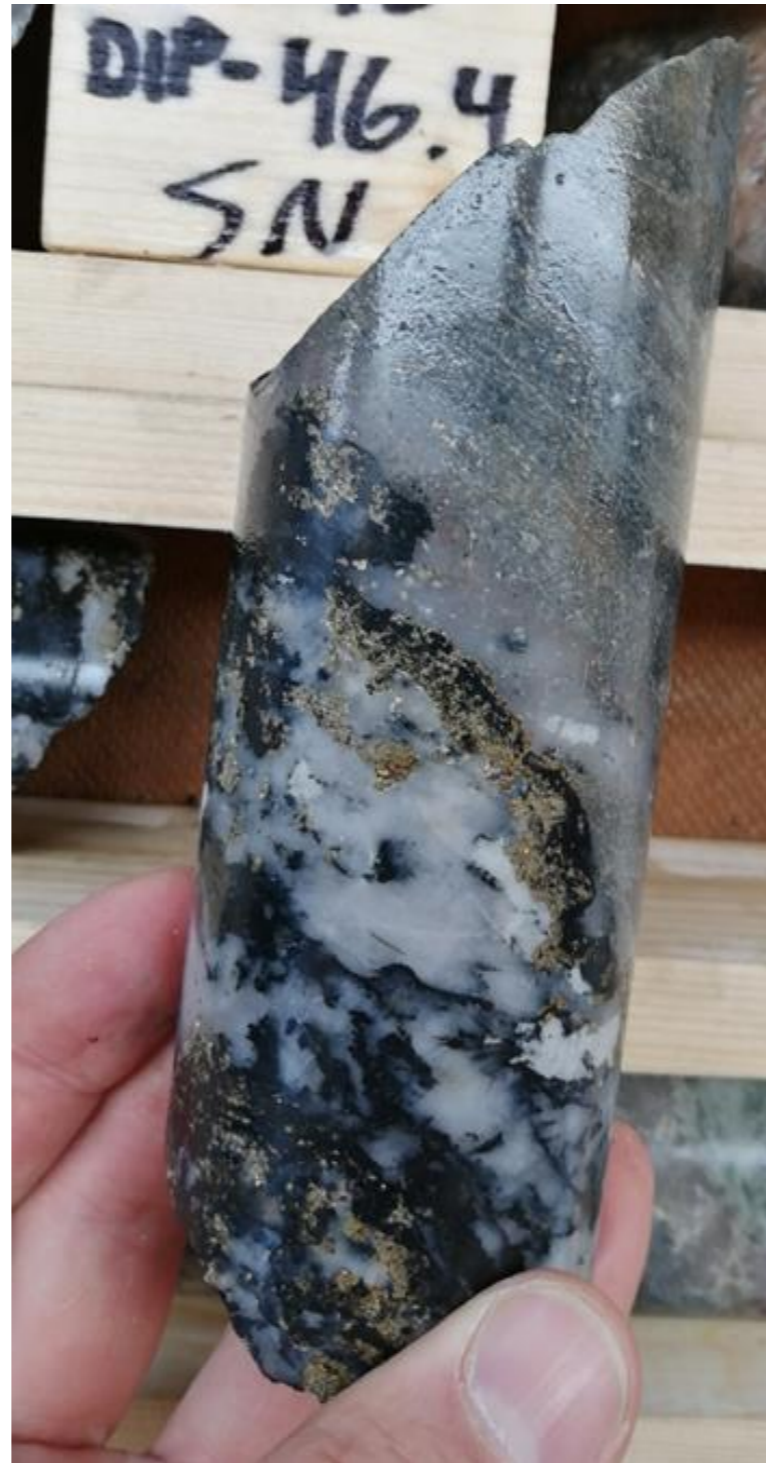
Drill hole 21MJ001. Left: QCTP Vein. Right: Visible Gold
