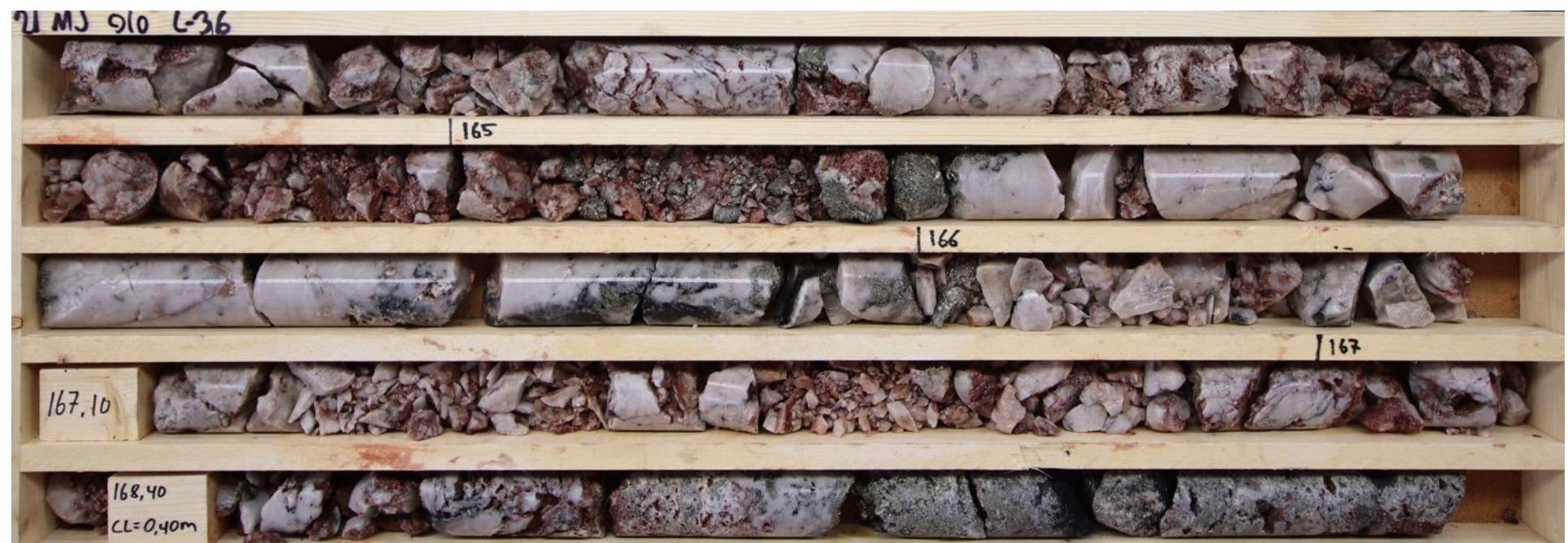
Drill hole 21MJ010. Above: Interval ~164.7-169.3m. Gold mineralized QCT veins including massive pyrite.
