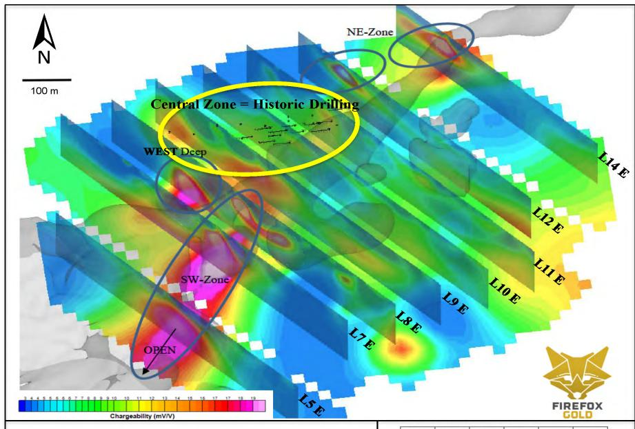
Mustajärvi IP Survey Summary: Vertical sections of chargeability together with horizontal chargeability section from 200 m depth. In addition, 3D-magnetic inversion bodies (grey) and shallow historical drill holes are shown.
